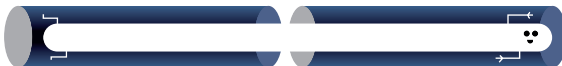
Cooper pairs can behave as if they were all a single particle that fills the entire electrical circuit. Quantum mechanics describes this collective state using a shared wave function . The properties of this wave function play the leading role in the laureates' experiment.
