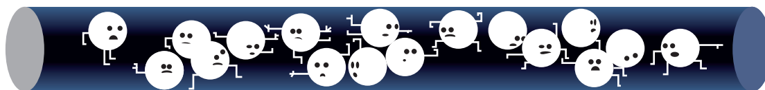
In a normal conductor, the electrons jostle with each other and with the material.
