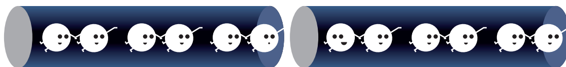
When a material becomes a superconductor, the electrons join up as pairs, Cooper pairs , and form a current where there is no resistance. The gap in the illustration marks the Josephson junction.
