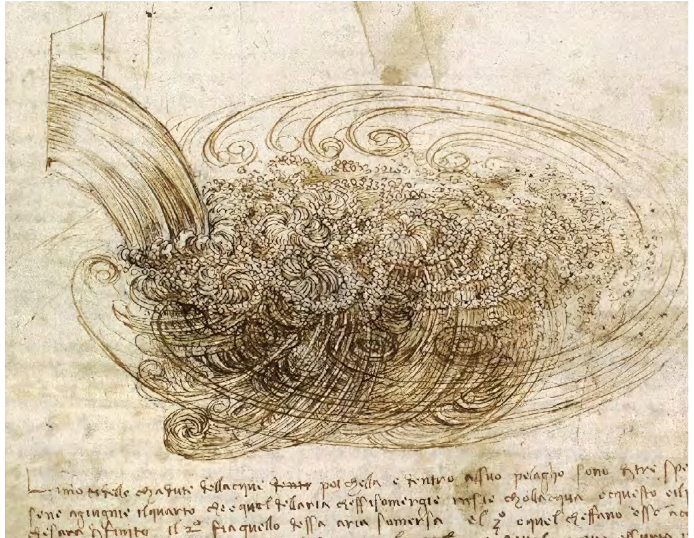
Fig. 1. Leonardo da Vinci's studies of water (c.1510-12). The fall of a stream of water from a sluice into a pool. This drawing depicts turbulence as composed of several eddies or vortices of different size, a quintessential feature of turbulence that several centuries later was formalized by the great mathematician Alexander Kolmogorov in what is now known as the cascade model of turbulence. But this was not the only attempt to represent this phenomenon mathematically. Later came the Navier-Stokes equation that models the dynamics of a fluid. This equation is essential to model the weather, blood flows, and the flying of airplanes, and yet it remains a mystery, as it has not been proved that it has a solution nor that this is unique, but it works!
