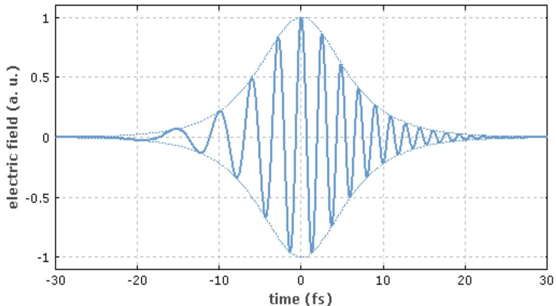
**Figure 4.** Chirped optical pulse, with the electric field plotted against time. The chirp of the pulse is the time dependence of its instantaneous frequency. The pulse is up-chirped, which means that the frequency increases with time. (Reproduced from <http://rp-photonics.com/chirp.html>.)
