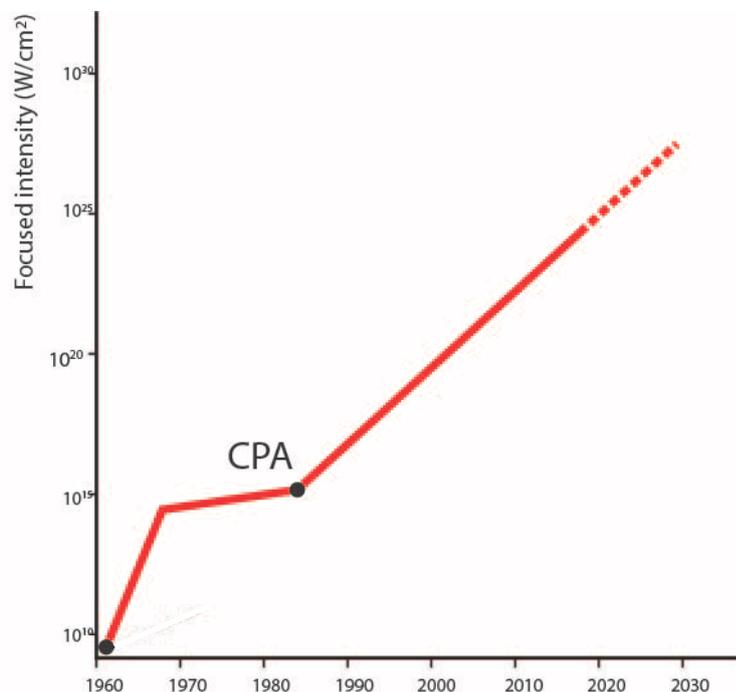
**Figure 3.** The history of pulsed laser technology in terms of peak intensity. After an initial increase in intensity during the 1960s, as described in the text, only an incremental increase occurred during more than a decade. The invention of the CPA technique for optical pulses by Strickland and Mourou in 1985 [45] dramatically changed the situation. The values on the y-axis are indicative because the intensity depends on how sharply the laser beam is focused.
