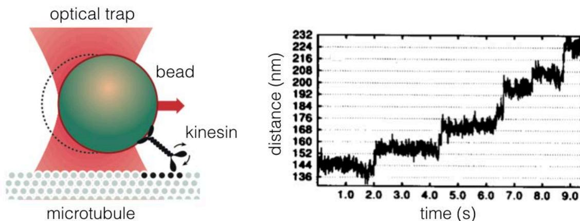
**Figure 2:** (Left) Sketch of the kinesin-microtubule system studied with optical tweezers in reference [39]. An optically trapped bead carries a single kinesin molecule that walks along an immobilized microtubule filament. (Right) Displacement versus time graph for a bead, which shows that the kinesin molecule executes a walk, pulling the bead forward in a stepwise manner. Sources: reference [39].
