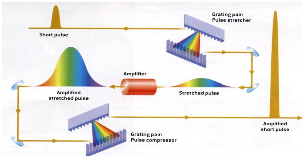
**Figure 5.** The standard CPA configuration. The chirp is illustrated with colours. Initially the gain medium (amplifier) was Nd:glass, whereas today, another common gain medium is Ti:sapphire. (Reproduced from Center for Ultrafast Optical Science, University of Michigan in Ann Arbor.)
