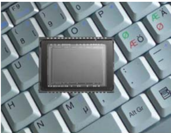
Fig. 6. A multi-megapixel camera CCD chip.
